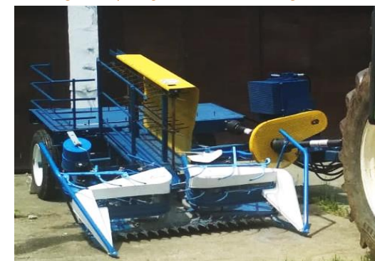
Fig.2 - Innovative Technical System for Harvesting Hemp Stalk, SRC-0
